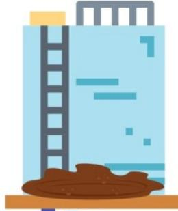
2. The water slows down and allows the dirt to settle to the bottom of the tanks. It is then filtered.
